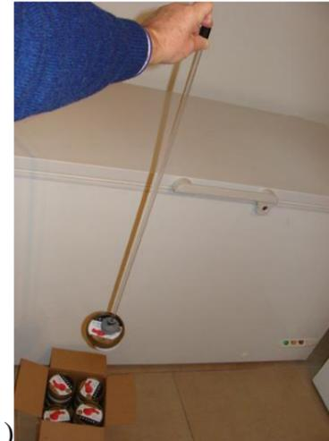
For products that rest deeper, use the hand gripper (Fig. 2.1)
