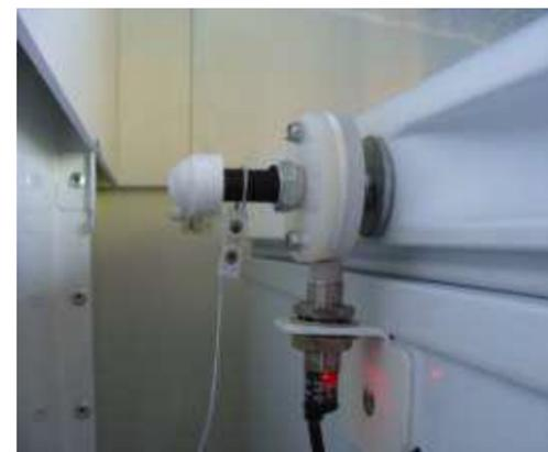
Fig. 1.4 b Sensor of 'freezer closed'
